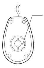
The 'ARROW' shows the unlocking direction. Lock by pushing the 'ARROW' in the opposite.
